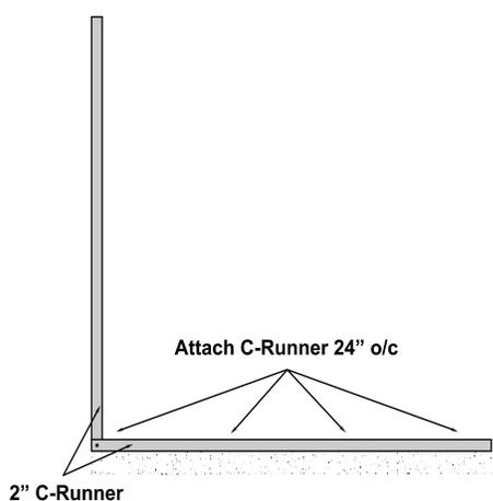
At the base, attach the 2" C-Runner track with proper fasteners spaced 24" o/c
