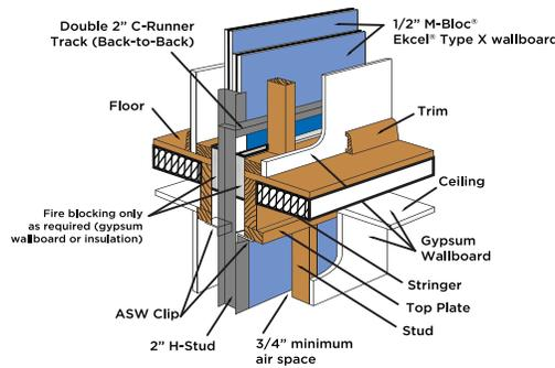
**Intermediate Floor Intersection / Trusses**
