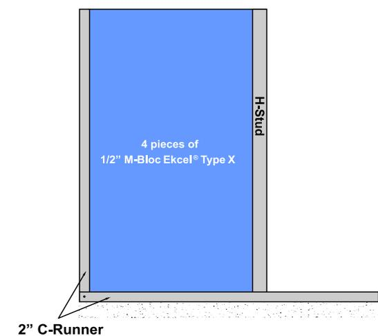
Finish off that section with a 4th and final panel, making sure only full-length panels are used. Ensure that all pieces of 1/2" M-Bloc Ekcel® Type X Wallboard are seated properly and that their edges are flush. Then insert a vertical H-Stud into the 2" C-Runner track and engage the H-Stud legs over the exposed long edges of the M-Bloc Ekcel® panels. Seat the H-Stud fully so the wallboard edges contact the stud web.
