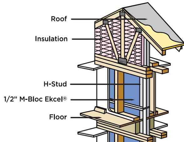
**Preserving Fire Rating in Attic Area with Insulation**
