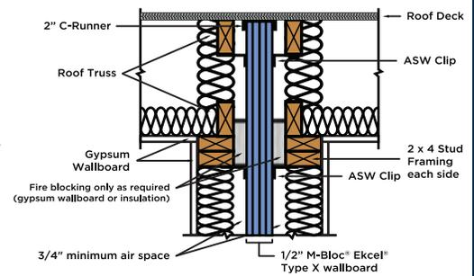
**Typical Roof Parapet Detail**
