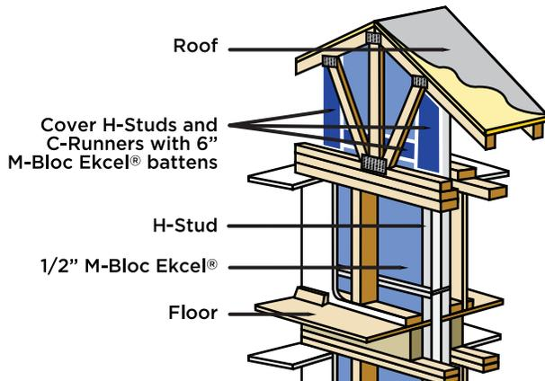
**Preserving Fire Rating in Attic Area with M-Bloc Ekcel Batten Strips**
