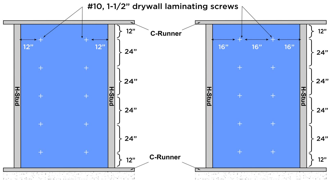
Laminating Screws - Once erected, the 4 pieces of 1/2" M-Bloc Ekcel® Type X Wallboard are secured to each other between H-Studs, with #10, 1-1/2" drywall laminating screws - from both sides of the wall.
