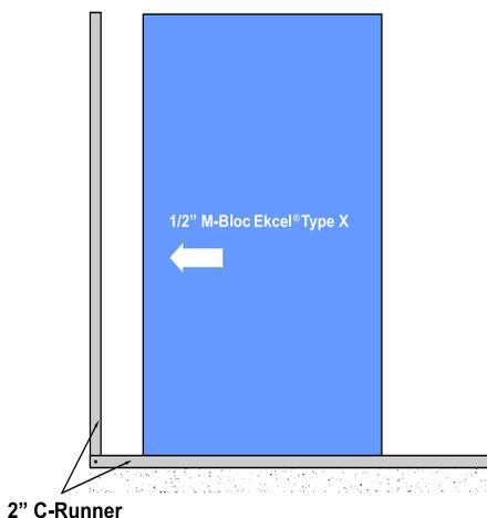
Insert a piece of 1/2" M-Bloc Ekcel® Type X Wallboard into the 2" C-Runner track.
