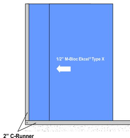
Once the 1st panel is in place, insert the 2nd piece of 1/2" M-Bloc Ekcel® Type X Wallboard, then the 3rd panel.
