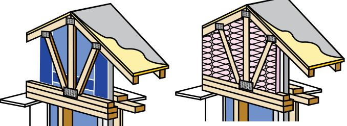
The 2" x 4" wood framed flanking wall, parallel to the ME Area Separation Firewall system may be oriented with nominal 2" face of the stud perpendicular to the four pieces of 4' wide, 1/2" M-Bloc Ekcel® Type X Wallboard with Mold & Moisture Resistance
