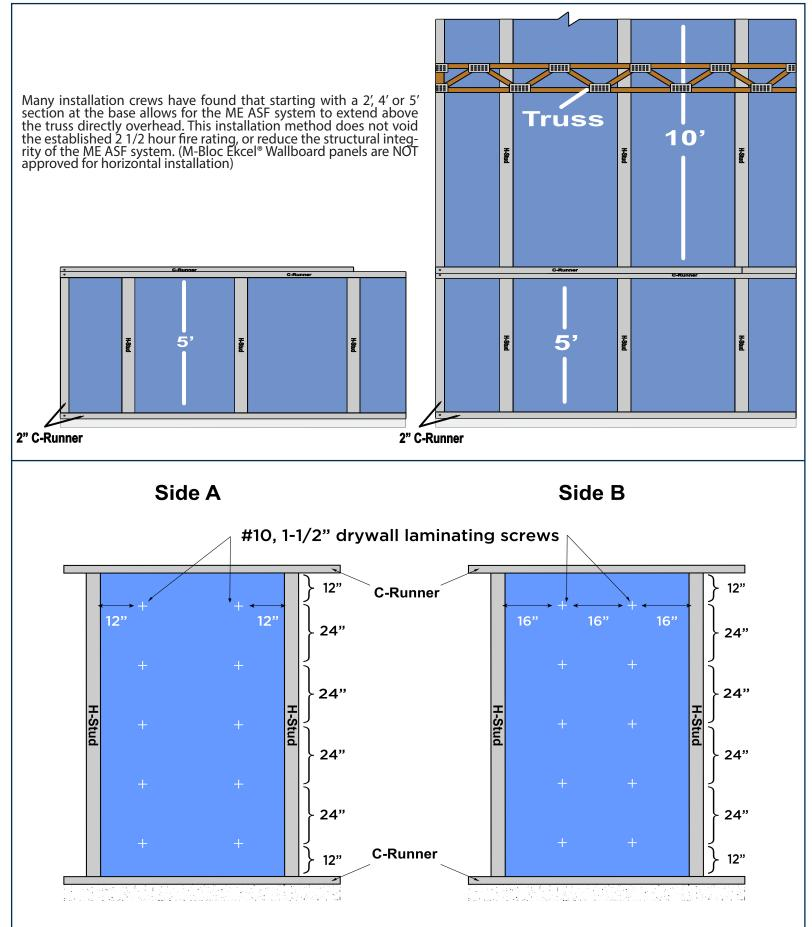
Laminating Screws - Once erected, the 4 pieces of 1/2" M-Bloc Ekcel® Type X Wallboard are secured to each other between H-Studs, with #10, 1-1/2" drywall laminating screws - from both sides of the wall.
